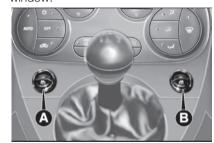
Hold the button pressed for a few seconds to wind the window down automatically or hold it pressed to wind the window up automatically (with the key at MAR only).
