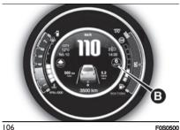
In AUTO mode the system changes gear depending on the car speed, the engine rpm and the intensity with which the accelerator pedal is pressed. A gear change can be requested using the control lever without having to switch off this mode: this function. known as "gear suggestion", suspends the automatic mode for the time necessary to make the gear selection requested by the driver.
