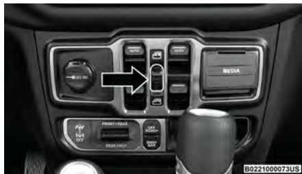
Window Lockout Switch
