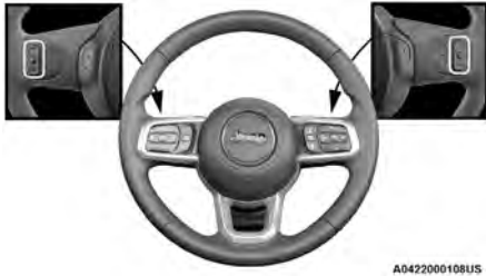
Remote Sound System Controls
