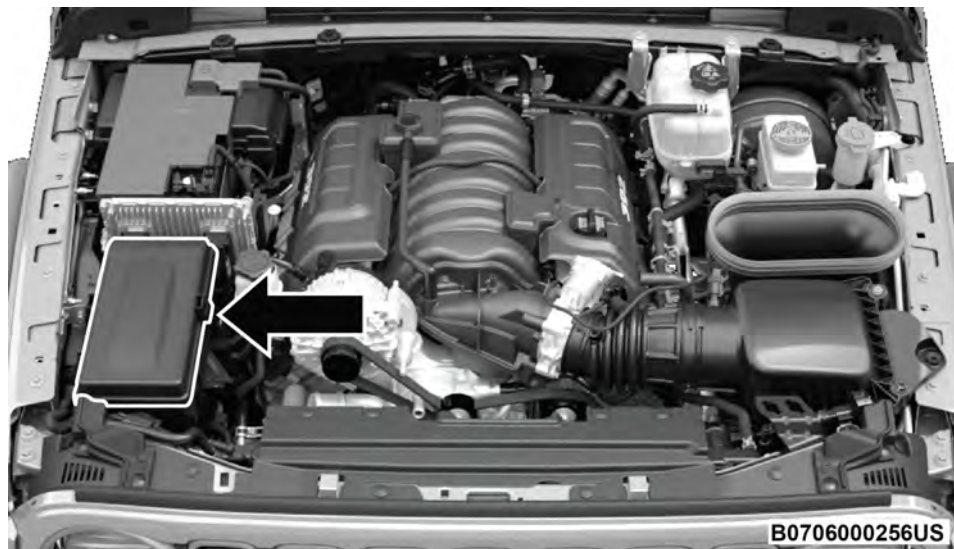
Power Distribution Center Location (6.4 Engine)
