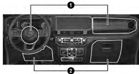
Front Air Bag/Knee Impact Bolster Locations
