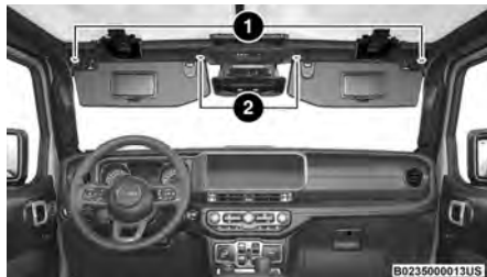
Interior Torx Screw Locations
