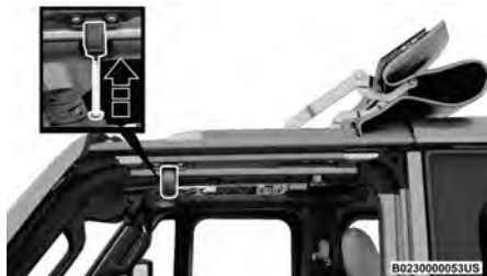
Attach Front Door Rail Bolt
