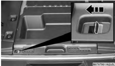
Hardware Storage Cover Latch
