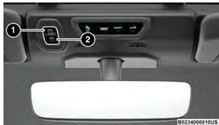
Power Sliding Top Control Switch
