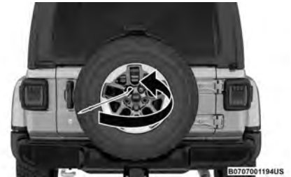
Removing The Spare Tire
