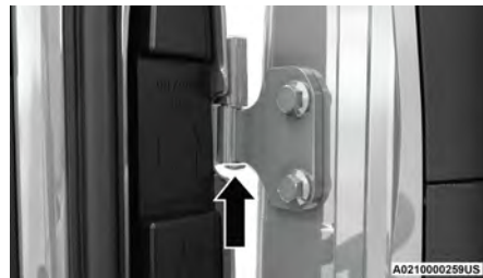
Hinge Pin Screw
