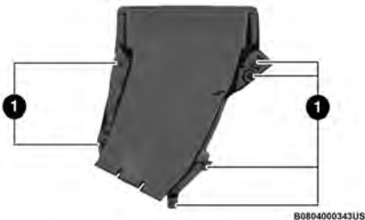
First Water Separation Chamber
