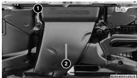
First Water Separation Chamber
