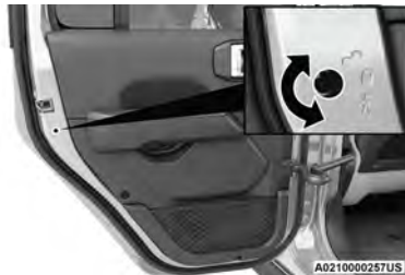
Child-Protection Door Lock Function
