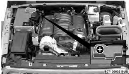
Positive (+) Battery Post (6.4 Engine)
