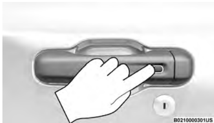
Push The Door Handle Button To Lock
