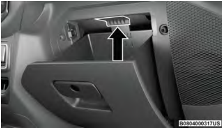
Glove Compartment Travel Stop
