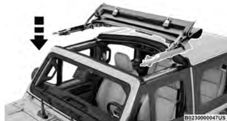
Lower Sunrider® Onto The Vehicle
