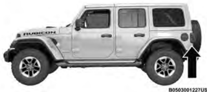
BSM Radar Location (Left Side Shown)
