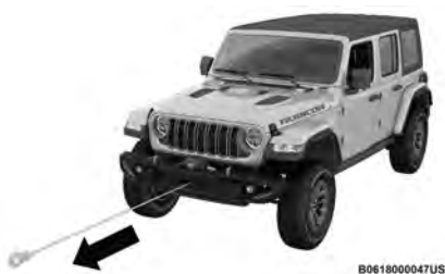
Pulling Synthetic Rope
