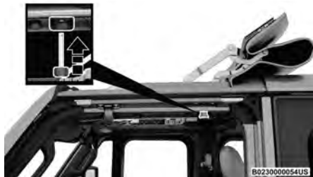
Attach Rear Door Rail Bolt
