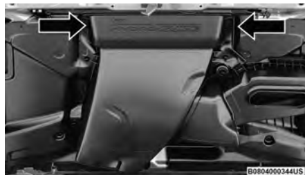
First Water Chamber Removal
