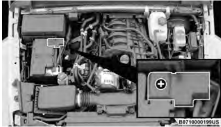
Positive (+) Battery Post
