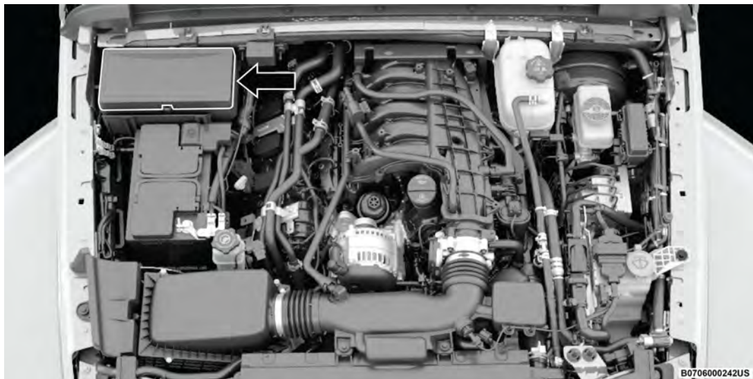
Power Distribution Center Location
