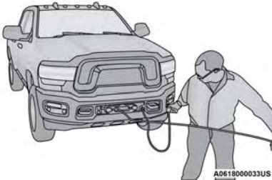
Pulling Synthetic Rope Under Tension
