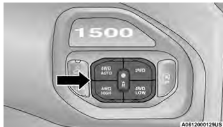
Five-Position/On-Demand Transfer Case — GT Models
