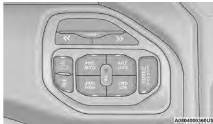
Four-Position/On-Demand Transfer Case
