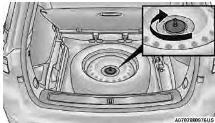
Reinstalling Tire Fastener
