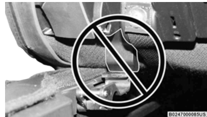
Incorrectly Seated Retainer
