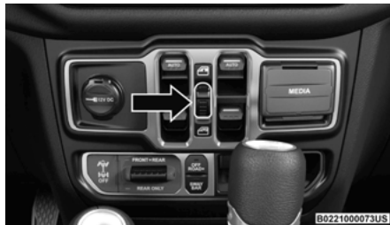
Window Lockout Switch
