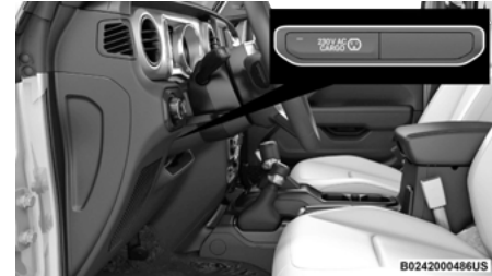
Power Inverter Switch (If Equipped)
