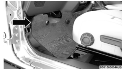
Front Carpet Pulled Away
