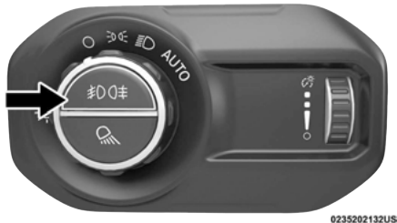
Fog Light Switch Location
